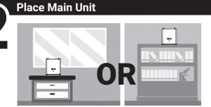
Place the Main Unit where signal exists (i.e. window). This will be the Donor Signal. Alternatively the Patch Antenna can be placed here, and the Main Unit can be placed at a distance.
