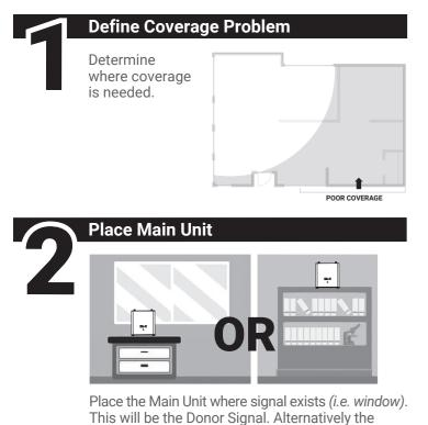
This will be the Donor Signal. Alternatively the Patch Antenna can be placed here, and the Main Unit can be placed at a distance.
