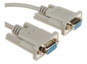
Maximum cable length is 15meters, or the cable length equal to a capacitance of 2500 pF (for a 19200 baud rate). Using lower capacitance cables can increase the distance. Reducing communication speed also can increase maximum cable length. The following table lists boud rate vs. Maximum cable length.
