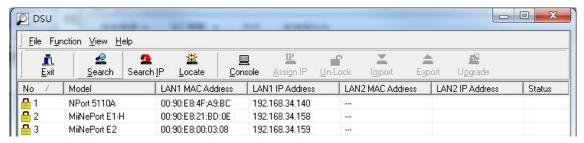
4. To modify the configuration of the highlighted MiiNePort E1, click the **Console** icon to open the web console. This will take you to the web console, where you can make configuration changes. Refer to **Chapter 7:** Web Console Configuration for information on how to use the web console.
