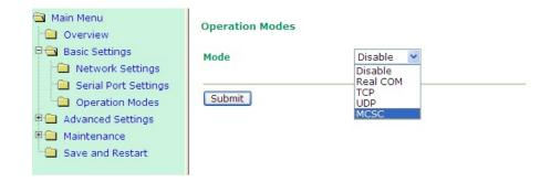
After **MCSC mode** is selected, you will see 2 channels that are ready to configured. Under the MCSC structure, each channel works independently so you need to configure each channel separately according to your application. Click **Modify** to configure the Channel 1.
