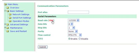
MiiNePort E1 supports the **Any Baud Rate (non-standard baud rate)** feature. If your baud rate is not listed, select **Other** from the drop-down list and type the baud rate in the input box. MiiNePort E1 will use the closest baud rate we can support.
