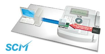
MiiNePort E1's SCM (Serial Command Mode) allows the module's parameters to be retrieved or configured through the serial port, rather than over the network. This is done through the use of specially parsed commands sent to the module through the serial port.
