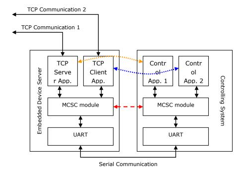
The MCSC module is built into the MiiNePort E1. To enable MCSC, you need to set your MiiNePort E1 serial port operation mode to MCSC mode and then set the channels' operation mode individually according to your application. In addition, you also need to implement the MCSC module in your device's main system.
