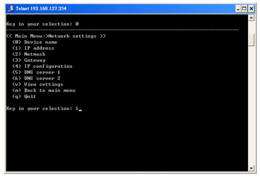
5. Use the backspace key to erase the current IP address. Type in the new IP address and then press **Enter**.
