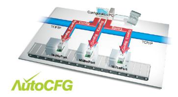
The MiiNePort E1's AutoCFG function is designed to allow users to realize true mass production. With AutoCFG, you no longer need to configure network modules one by one during the device manufacturing process. To use AutoCFG, follow the steps described below:
