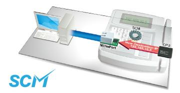
The MiiNePort E1/E2-SDK's SCM (Serial Command Mode) allows the module's parameters to be retrieved or configured through the serial port, rather than over the network. This is done through the use of specially parsed commands sent to the module through the serial port.
