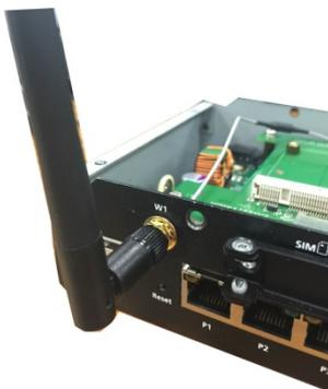
7. Reattach the cover on to the computer and fasten the screws to secure it in place.
