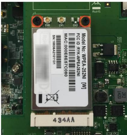
3. Attach one end of the Wi-Fi cable on the connector marked CH0, and then connect the other end of the cable on the W1 hole on the front panel of the computer. Remove the antenna hole protection cover before you do so.
