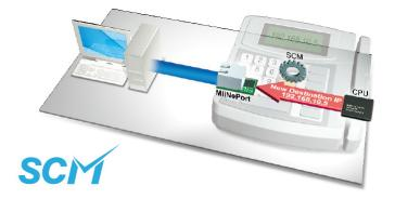
MiiNePort E1's SCM (Serial Command Mode) allows the module's parameters to be retrieved or configured through the serial port, rather than over the network. This is done through the use of specially parsed commands sent to the module through the serial port.
