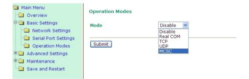
After **MCSC mode** is selected, you will see 2 channels that are ready to configured. Under the MCSC structure, each channel works independently so you need to configure each channel separately according to your application. Click **Modify** to configure the Channel 1.
